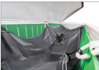
Geotextile bag effectively separates solids from water.
