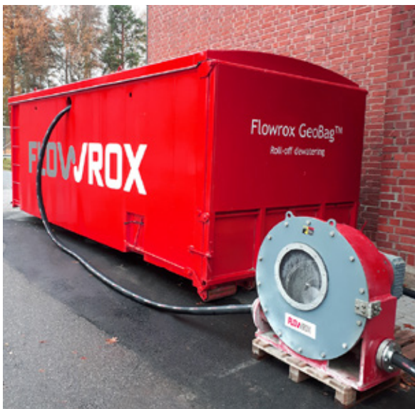
Outside view of Flowrox GeoBag™ with an LPP-T65 sludge transfer pump.
