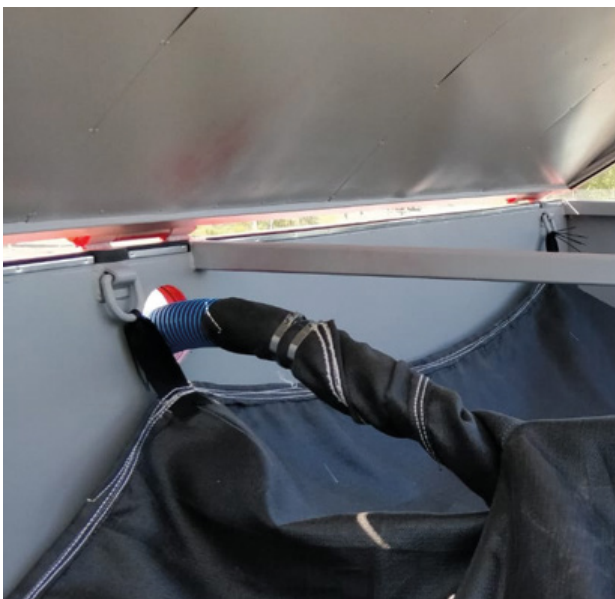
Geotextile bag sleeve is wrapped and fastened around the sludge inlet.
