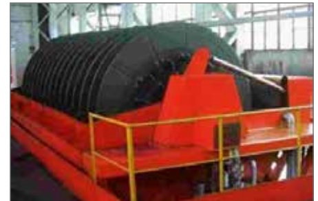
Capacity of Flowrox Ceramic Disc Filter is high: up to 2000 kg DS/m 2 per hour.
