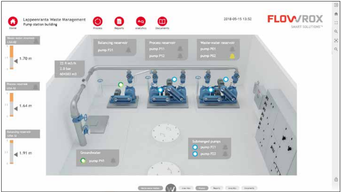
Remote, online view of Flowrox Malibu™: exact model of the real EKJH pump station.
