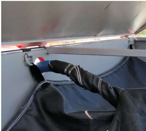
Geotextile bag sleeve is wrapped and fastened around the sludge inlet.
