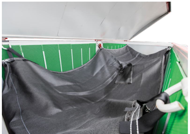
The geotextile filtration bag is mounted inside the container.
